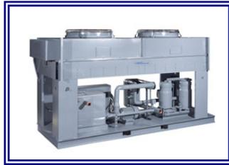
Cooling Technology's Air Cooled Chiller features an integral tank and pump. In addition the ICA houses a reciprocating or screw compressor paired with a stainless steel brazed plate evaporator and an integral MDPE reservoir with a non-ferrous pump. Our ICA line of chillers are available in 15 to 140 ton capacities.
